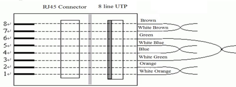
The RJ45 connect comply with TIA/EIA 568B standard.
